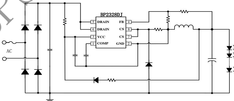
Figure 1. Typical application circuit for BP2328DJ
